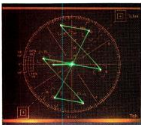
Figure 7. Color bars on a vectorscope.
